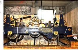
has a double 3-legged gravity escapement which is often used in large 'tower' clocks to produce a reliable and consistent push to keep the pendulum swinging accurately.
